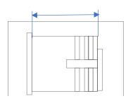
MINIMUN THICKNESS IS 25MM, WE CANNOT PROVIDE SHORTER CYLINDER; ADD CYLINDER COLLAR AS A SOLUTION Available size: 25/29/32/35/38/44mm
