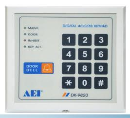
DK-9820 mainly designed for stand-alone electric door lock installation. Its 5 Amp output relay provides N.C. and N.O. dry contacts for door strike and virtually compatible with any electric locking devices. Except the inter-lock and door open/close monitoring facilities, the keypad has most of the basic features just like the other keypads in this series..
