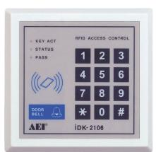
IDK-2106 mainly designed for stand-alone electric door lock installation. Its 5 Amp output relay provides N.C. and N.O. dry contacts for door strike and virtually compatible with any electric locking devices. Except the inter-lock and door open/close monitoring facilities, the keypad has most of the basic features just like the other keypads in this series..
